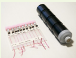
Pinger ultrasonic tag and receiver
