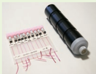
Pinger ultrasonic tag and receiver
