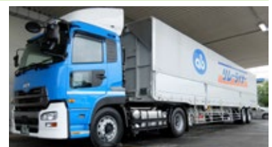
Specialty-designed trailer Relay Liner® Loads 1.5 times the pallets of a regular truck (16 pallets increased to 24)
