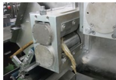
Simulating a caught-in accident in a rolling machine (Ajinomoto Frozen Foods Co., Inc.)
