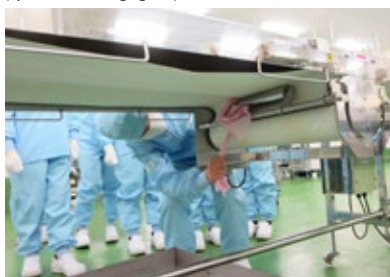
Simulating getting caught in a conveyor roller (Ajinomoto Frozen Foods Co., Inc.)
